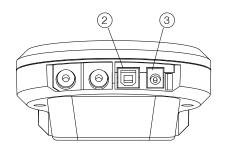
(1) Banana plugs for transmitter connection | (2) USB 2.0 port | (3) Battery charger connection
