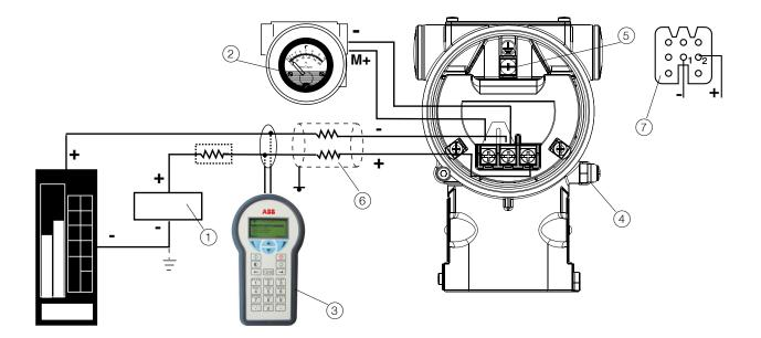
1 Power source | 2 Remote indicator | 3 Handheld communicator | 4 External ground termination point | 5 Internal ground termination point | 6 Line load | 7 Harting Han 8D socket insert for mating plug (supplied loose)
